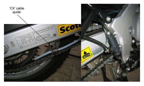
The dispenser head should be angled such that the slash cut dispenser is away from the sprocket and can drip oil onto the chain. If you turn it around it will pick up dirt off the sprocket & get blocked.
