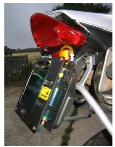
Fix an aluminium backing plate to the HCR itself and the lot was then assembled to the number plate holder to make the good stiff mounting, suffice to support the weight of the filled HCR.
