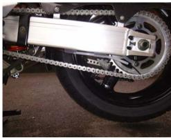
The Dispenser Assembly, shown left, is routed along the underside of the Swingarm using Dispenser Mounting Sleeves & Glue. **Note:** an epoxy resin (eg. Araldite) is req'd to bond the sleeves to the Swingarm.
