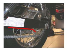
The Dispenser Assembly can be routed along the underside of the Swingarm, shown left, using Dispenser Mounting Sleeves & Glue. **Note:** an epoxy resin (eg. Araldite) is req'd to bond the sleeves to the Swingarm.
