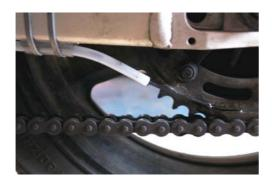
Once fitted, fill and prime the system and set the adjuster knob to 'prime'.
