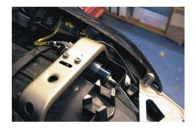
The Dispenser Assembly, shown bottom left, is routed along the underside of the Swingarm using Dispenser Mounting Sleeves, Cable Ties & Glue. **Note:** an epoxy resin (eg. Araldite) is req'd to bond the sleeves to the Swingarm.
